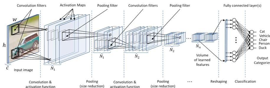
**Fig. 2.** Convolutional Neural Network for classification.
